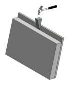
Adhesion to the formwork should be minimised before lifting the concrete element out of the formwork by removing as many parts of the formwork as possible.
