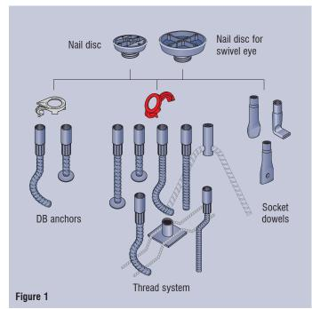
The plastic nail discs are used for the simple fastening of PFEIFER threaded anchors to the formwork.
