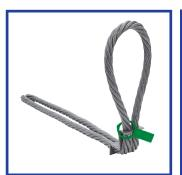
The PFEIFER Bent Loop was developed to be used as a lifting anchor for lifting concrete elements. Regular stresses are straight pull, parallel shear pull and transversal shear pull. The shape and the form of the holding bracket enable very simple installation and easy fixing to the reinforcement. Once the concrete has cured, a suitable suspension hook can be hooked into the protruding loop and the element can be transported safely.
