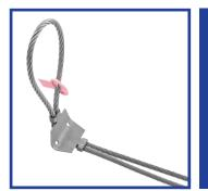
The PFEIFER Bent Loop was developed to be used as a lifting anchor for lifting concrete elements. Regular stresses are Advantages: straight pull, parallel shear pull and transversal shear pull. The shape and the form of the holding bracket enable very simple installation and easy fixing to the reinforcement. Once the concrete has cured, a suitable suspension hook can be hooked into the protruding loop and the element can be transported safely.
