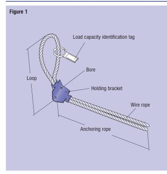
PFEIFER Bent Loops consist of a specially shaped holding bracket, a high-quality rope and an appropriately marked load capacity tag.
