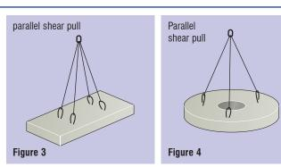
The PFEIFER bent loop is intended for the lifting and transport of plane precast units. In regular use the bent loops may be loaded straight or up to an angle of inclination of 30° from the perpendicular only in the direction of the free rope ends.
