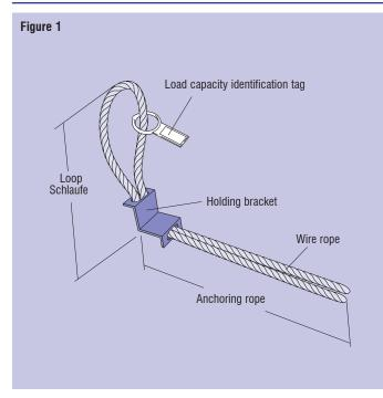
PFEIFER bent loops consist of a specially shaped holding bracket, a highquality rope and an appropriately marked load capacity identification tag. The holding bracket is intended for the correct alignment of the loop and for fixing to the reinforcement with wire or cable ties. The free ends are for anchoring in the concrete. In the cast in concrete state, the loop protrudes above the concrete surface and can be used for attachment when lifting or transporting the precast concrete element.
