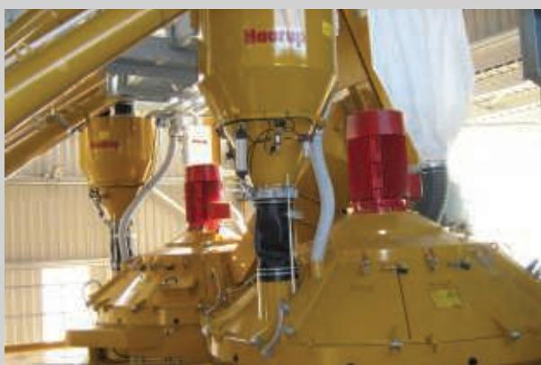
Cement weigh hoppers suspended in electronic load cells.
