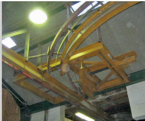
Switch-track for mono-trans concrete travelling bucket.
